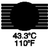
**High Temperature.** Depressing this switch will activate the unit to draw in room air, heat the air to 43.3°C +4.0°C/ -2.0°C and deliver it to the patient via the disposable blanket. The LED will be activated to indicate that the unit is in the high temperature mode. **The high temperature setting is to be used with close patient observation.**
