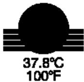
**Medium Temperature.** Depressing this switch will activate the unit to draw in room air, heat the air to 37.8°C +4.0°C/ -2.0°C and deliver it to the patient via the disposable blanket. The LED will be activated to indicate that the unit is in the medium temperature mode.
