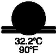
**Low Temperature.** Depressing this switch will activate the unit to draw in room air, heat the air to 32.2°C +4.0°C/ -2.0°C and deliver it to the patient via the disposable blanket. The LED will be activated to indicate that the unit is in the low temperature mode.
